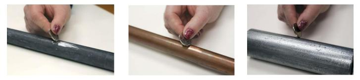
Lead pipes will turn a shiny silver when scratched by a coin. Copper pipes will turn shiny like a new penny. Steel pipes will maintain their color.
