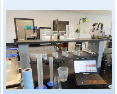
The above picture represents one of the small items needing completion at both plants. That is testing the dosage strength of coagulants/polymer's used to create floc at the water plant to settle out dirt from the water. And to dewater sludge at the wastewater plant to create a drier sludge cake for transportation to the landfill.
